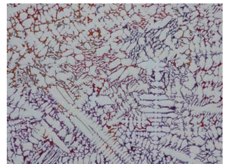
Brass as cast etched with Klemm III 10x. Prepared according to SumMet method using CarbiMet abrasive papers.
